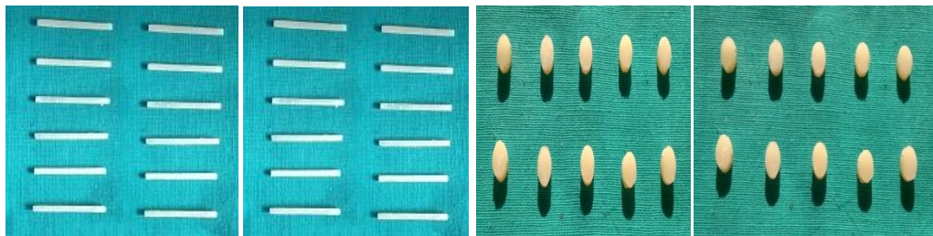
Figure 2 a) Group I. Flexural strength specimen (self cure) (b) Flexural strength specimen (dual cure) (c) Microhardness specimen (self cure) (d) Microhardness specimen (dual cure)
