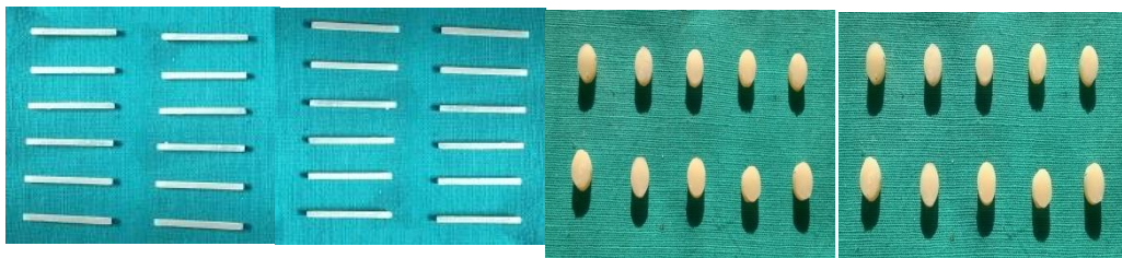
Figure 3 a) Group II. Flexural strength specimen (self cure) (b) Flexural strength specimen (dual cure) (c) Microhardness specimen (self cure) (d) Microhardness specimen (dual cure)
