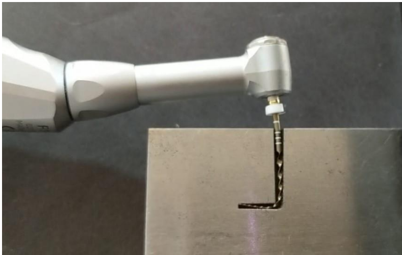
Fig 2: Experimental set up of the endomotor and metal block with 90° curvature with ProTaper Gold file
