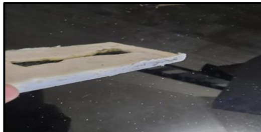
Figure 8. HDPE HDPE Reinforcement carbon fiber composite
