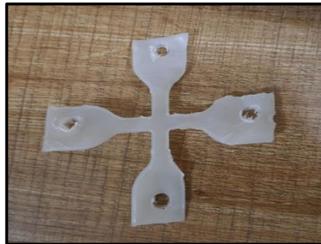
Figure 7. HDPE Sample cutting by lazer CNC
