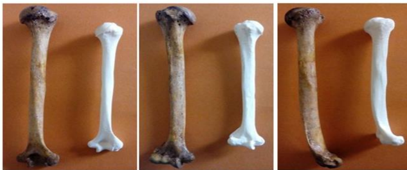
Figure 13 Posterior, anterior and side view of 3D printed reshaped bone and humerus bone
