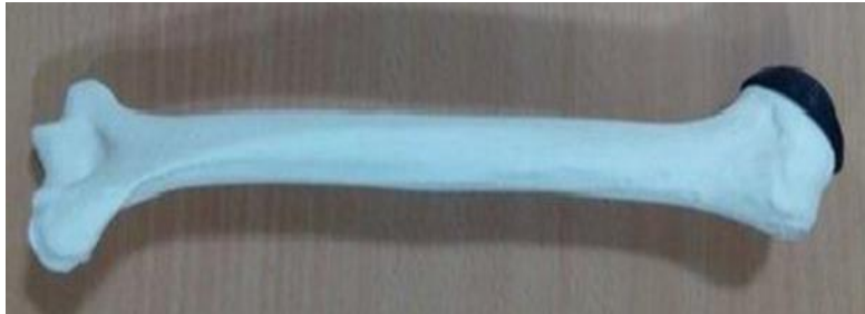
Figure 14 Assembled 3D printed humerus bone with proximal implant prototype
