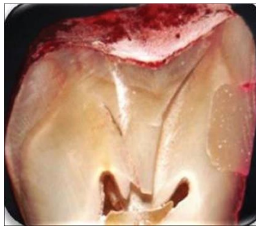
Figure 2. Dye penetration along the occlusal/gingival wall to less than half of the cavity depth (score 1)
