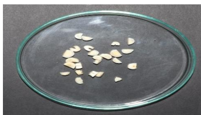
Fig. 2: Each dentin disc was divided into two halves to obtain 24 specimens
