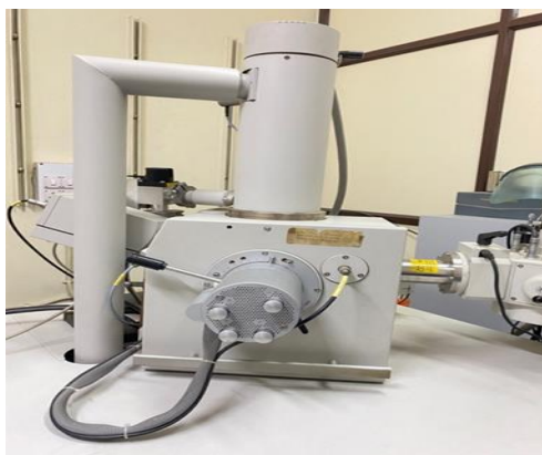
Fig. 5: SEM equipment (Jeol JSM-7600F) for observation of dentinal tubular occlusion
