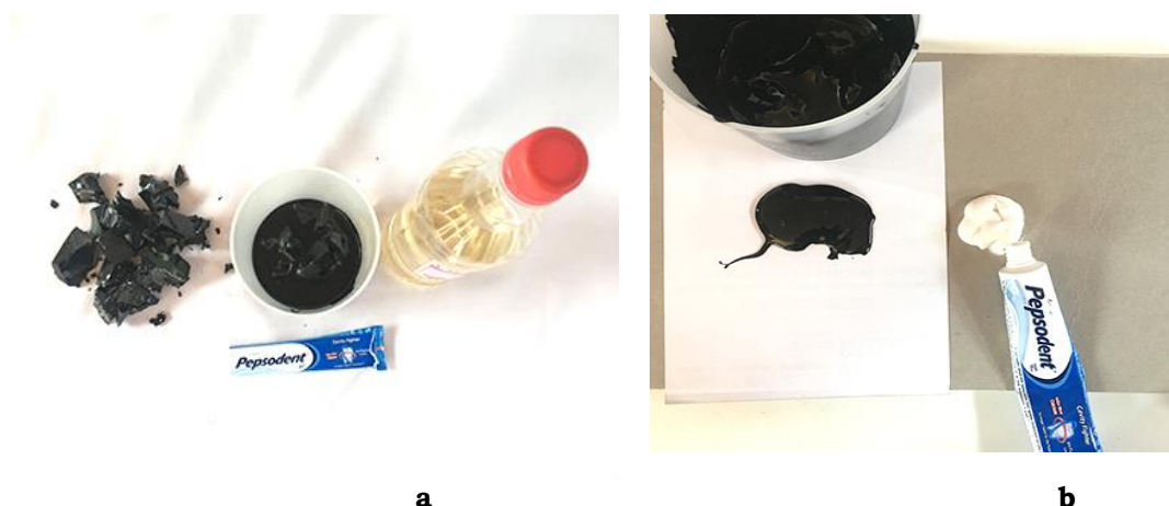
Figure 3 (a, b) Matching the dissolved asphaltum in turpentine with the consistency of tooth paste.
