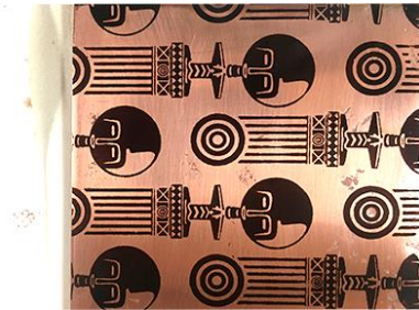
Figure 11 Square edge blade gave the best print with a crisp effect and better in definite edges of the motifs or designs printed.
