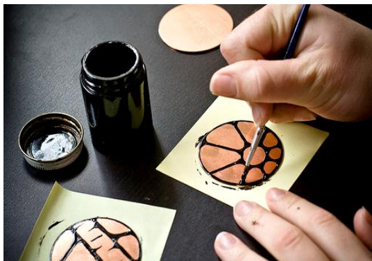
Figure 1 Applying resist with a sable brush (Source: Ganoksin, 2018).
