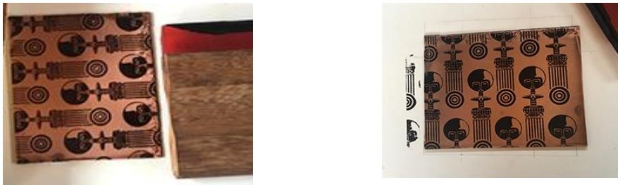
a - effect from bevelled edge blade b - effect from chamfered edge blade
