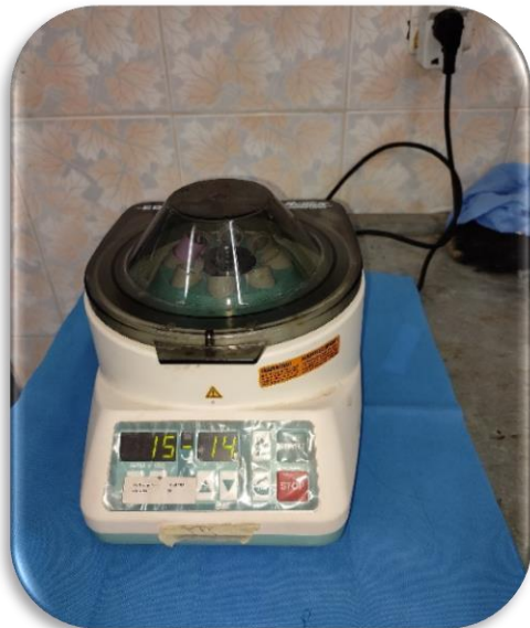
Figure 2a: centrifugation the blood sample with 1500 round per 14 mints
