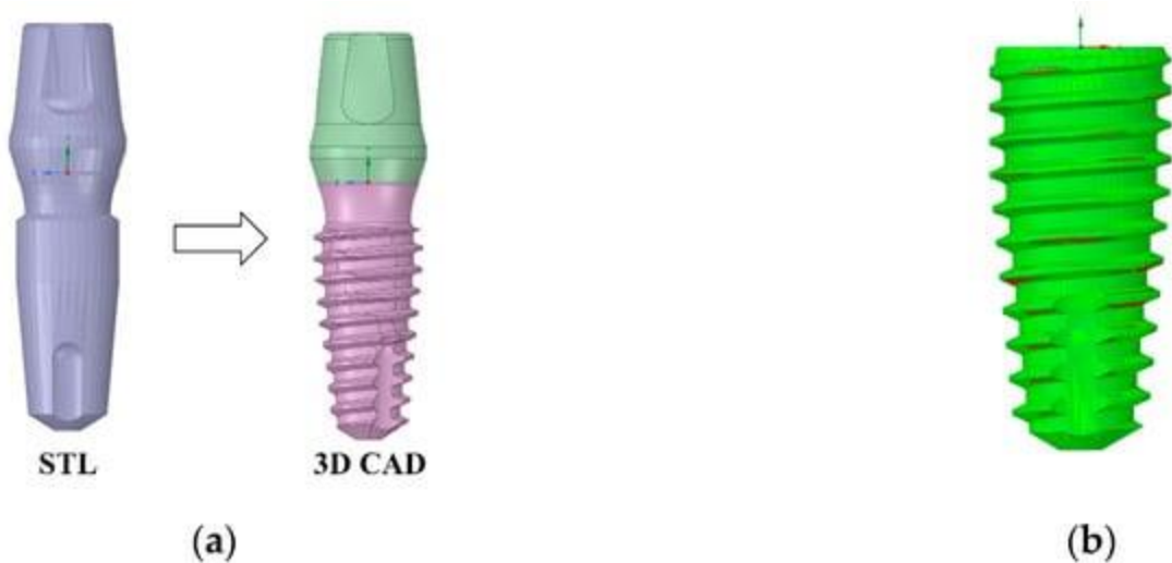
Figure 8. (a) STL to 3D CAD reverse engineering process; (b) in red, the deviation between the reconstructed geometry and the original STL file equals to 0.03 mm.
