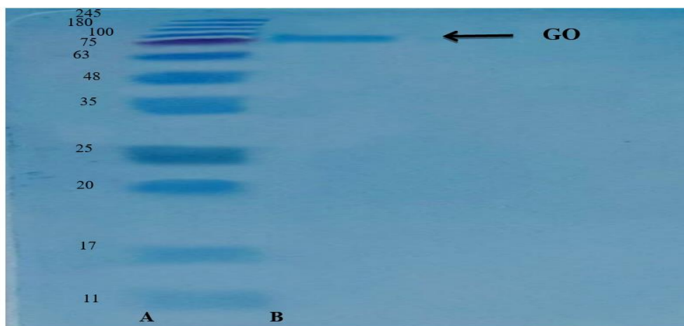
Figure(3) Electrophoresis of GOX enzyme in a polyacrylamide gel in the absence of teratogens. A represents the standard marker, known molecular weights, and B is A purified GOX enzyme.
