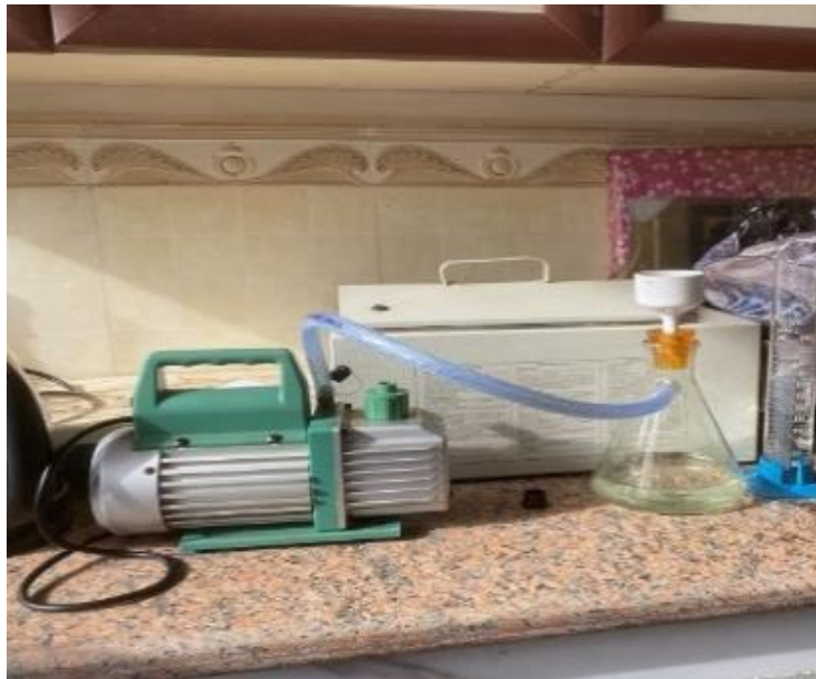
Figure 2. Filtering the sample using a microfiber filter
