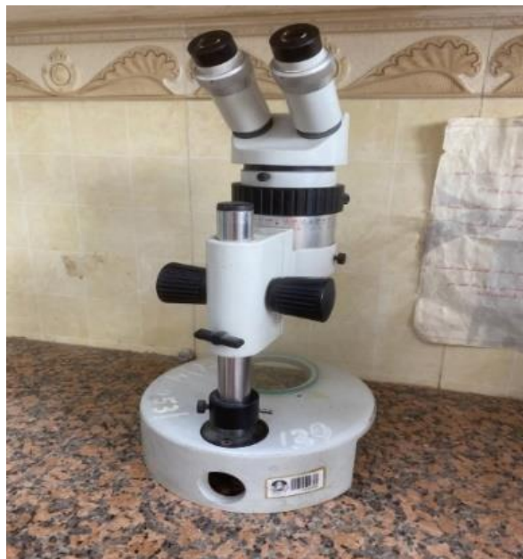
Figure 4. Determination of microplastic using a MOTIC-type anatomical microscope
