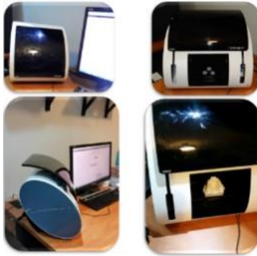
Figure 1: Photograph of a desktop Red Laser 3Shape D500 scanner
