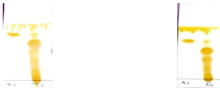
Figure 3 Thin layer chromatographic pattern of 70% methanol E.officinalis extract by maceration method (3a) and ethyl acetate fraction (3b). Chloroform: ethyl acetate: formic acid (2.8: 2.4: 0.4ml) used as a mobile phase solvent system. TLC plate exposed to iodine fumes. S1 and A1 are indicate ethyl gallate standards and, T1 is 70% methanol extract and B1 is ethyl acetate fraction.
