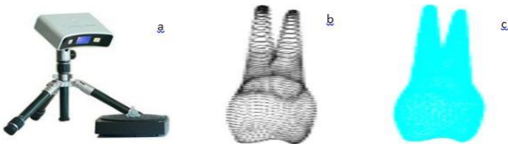
Figure. 1: (a) Laser scanner; (b) scanned tooth as a cloud of points; (c) scanned tooth after creating its surface
