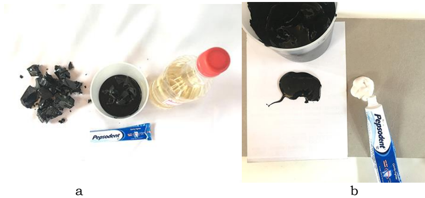
Figure 3. (a, b) Matching the dissolved asphaltum in turpentine with the consistency of tooth paste
