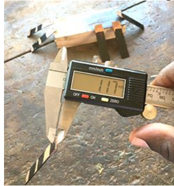
c - .2mm is an ideal layer to asphaltum resist a non-violent etchant Figure 5. Covering metal plate with asphaltum
