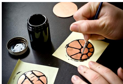
Figure 1. Applying resist with a sable brush Source: Ganoksin, 2018 & hand-drawn
