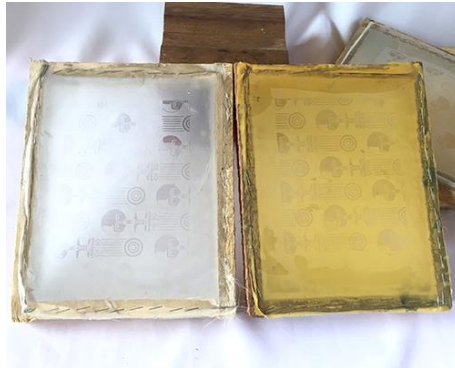
a - Left: shows a 'Normal Mesh', with between 40-86 mesh count, Right: 'Fine Mesh' with between 120-156 mesh count
