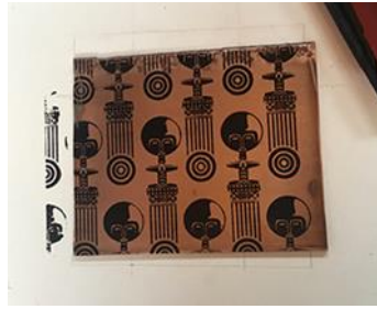
b - effect from chamfered edge blade Figure 9. Print effects from bevelled and chamfered edge squeegee type
