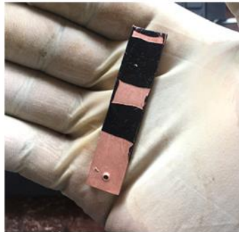
d - clean accurate edges in etching
