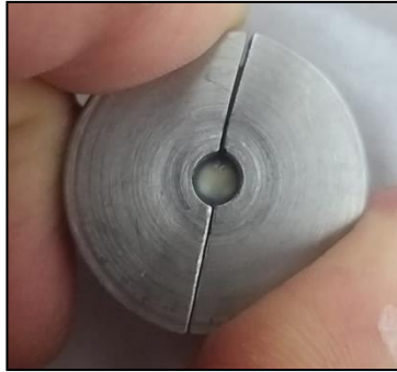
Figure 3. Metal matrix mold for applying composite resin
