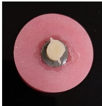
Figure 4. Sample bonded with repair material
