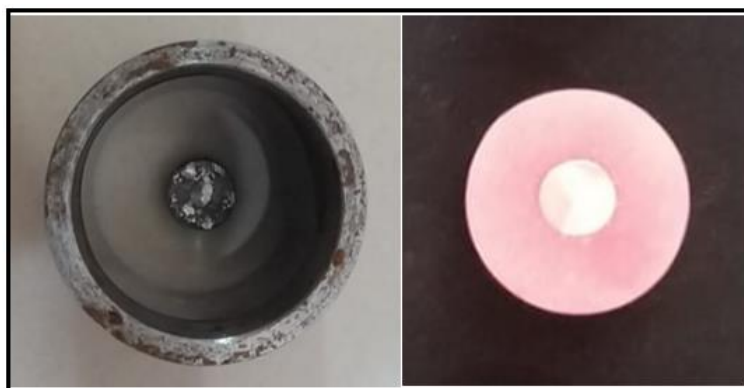
Figure 2. Sample embedded in an autopolymerized acrylic resin with the help of a metal jig
