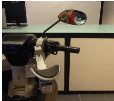
Figure 2: Prototype (armrest) attached to motorcycle's handle
