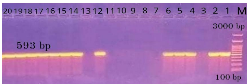
Figure 2: PCR results for the chromosomal algD gene, the electrophoresis done on agarose gel, 1.5% concentration, 70 volts, for an hour. The column M represents the ladder, while columns 1-20 represent the isolates.
