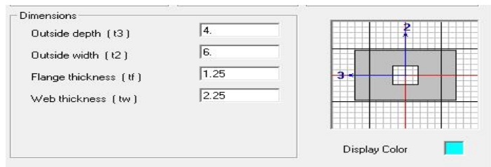
Fig 4 Pylon Bottom Frame Properties
