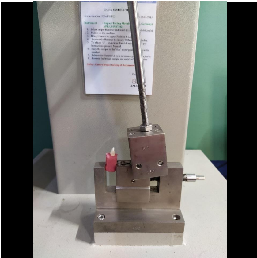
Figure 4. sample testing for impact fracture strength
