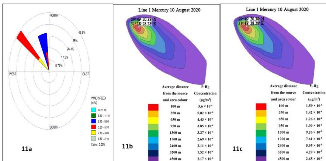
Figure (11): Output of the AERMOD model of line 1 in Helwan area during the day of sampling (August 10th, 2020) 11a (Wind speed (m/sec) and direction), 11b (Dispersion model of Particulate Mercury emission load in line 1), and 11c (Dispersion model of Vapour Mercury emission load)
