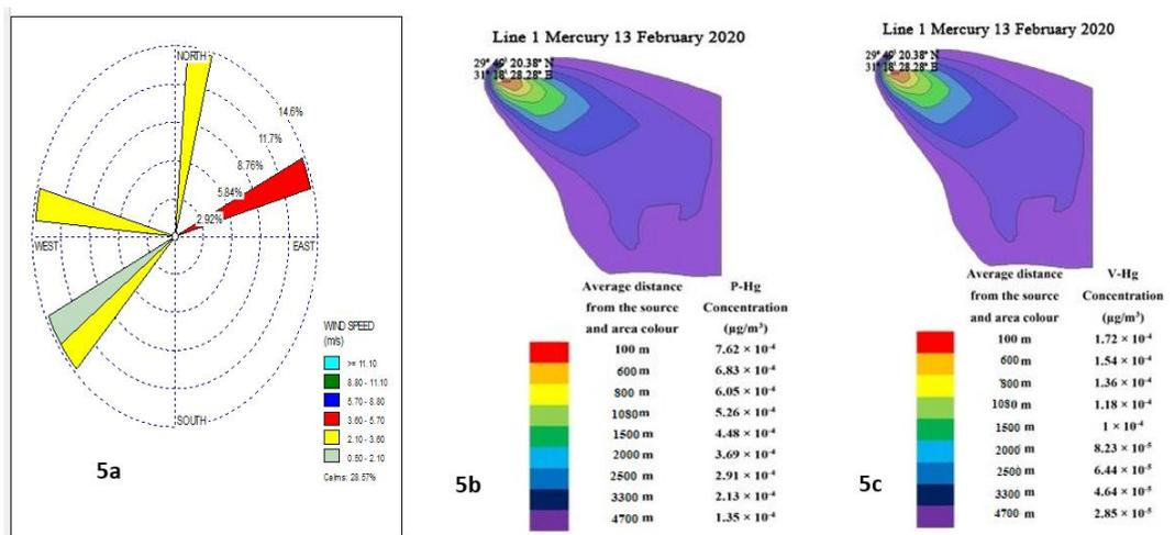
Figure (5): Output of the AERMOD model of line 1 in Helwan area during the day of sampling (February 13th, 2020) 5a (Wind speed (m/sec) and direction), 5b (Dispersion model of Particulate Mercury emission load in line 1), and 5c (Dispersion model of Vapour Mercury emission load)
