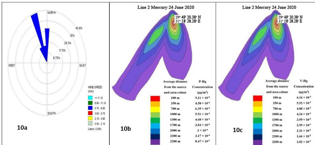
Figure (10): Output of the AERMOD model of line 2 in Helwan area during the day of sampling (June 24th, 2020) 10a (Wind speed (m/sec) and direction), 10b (Dispersion model of Particulate Mercury emission load in line 2), and 10c (Dispersion model of Vapour Mercury emission load)
