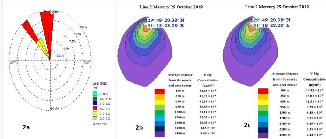
Figure (2): Output of the AERMOD model of line 2 in Helwan area during the day of sampling (October 29th, 2019)2a (Wind speed (m/sec) and direction), 2b (Dispersion model of Particulate Mercury emission load in line 2), and2c (Dispersion model of Vapour Mercury emission load)
