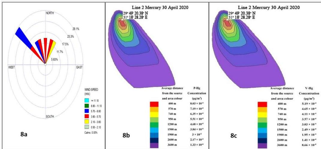
Figure (8): Output of the AERMOD model of line 2 in Helwan area during the day of sampling (April 30th, 2020) 8a (Wind speed (m/sec) and direction), 8b (Dispersion model of Particulate Mercury emission load in line 2), and 8c (Dispersion model of Vapour Mercury emission load)
