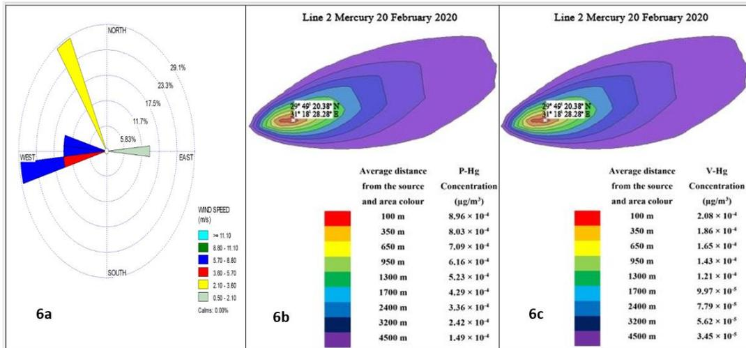
Figure (6): Output of the AERMOD model of line 2 in Helwan area during the day of sampling (February 20th, 2020) 6a (Wind speed (m/sec) and direction), 6b (Dispersion model of Particulate Mercury emission load in line 2), and 6c (Dispersion model of Vapour Mercury emission load)
