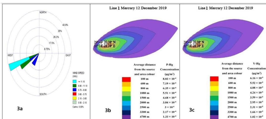
Figure (3): Output of the AERMOD model of line 1 in Helwan area during the day of sampling (December 12th ,2019) 3a (Wind speed (m/sec) and direction), 3b (Dispersion model of Particulate Mercury emission load in line 1), and 3c (Dispersion model of Vapour Mercury emission load)
