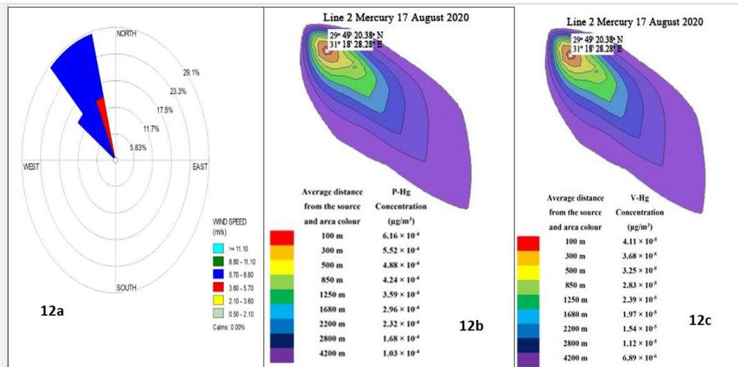
Figure (12): Output of the AERMOD model of line 2 in Helwan area during the day of sampling (August 17th, 2020) 12a (Wind speed (m/sec) and direction), 12b (Dispersion model of Particulate Mercury emission load in line 2), and 12c (Dispersion model of Vapour Mercury emission load)
