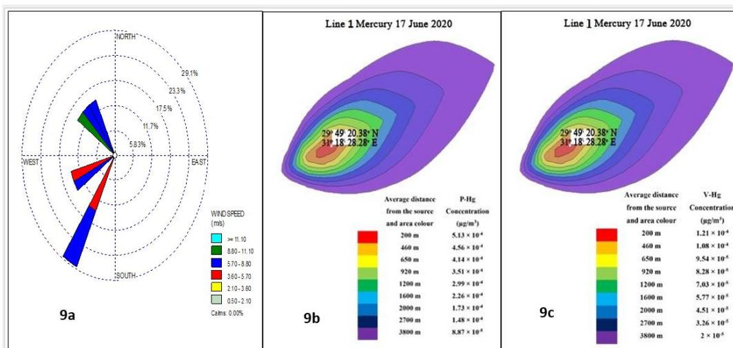
Figure (9): Output of the AERMOD model of line 1 in Helwan area during the day of sampling (June 17th, 2020) 9a (Wind speed (m/sec) and direction), 9b (Dispersion model of Particulate Mercury emission load in line 1), and 9c (Dispersion model of Vapour Mercury emission load)
