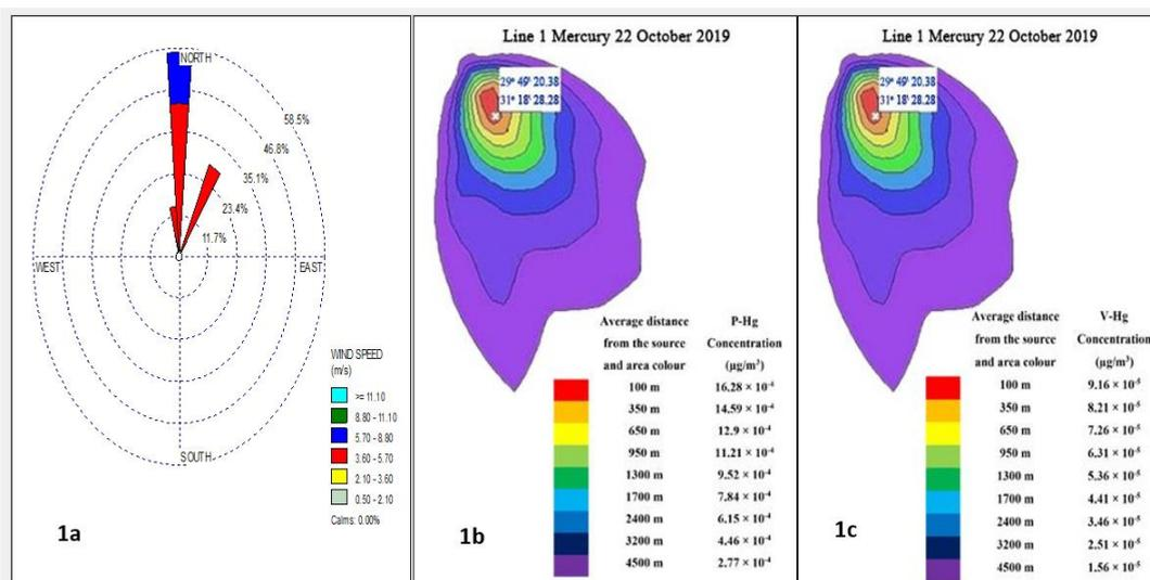
Figure (1): Output of the AERMOD model of line 1 in Helwan area during the day of sampling (October 22nd, 2019) 1a (Wind speed (m/sec) and direction), 1b (Dispersion model of Particulate Mercury emission load in line 1), and 1c (Dispersion model of Vapour Mercury emission load)
