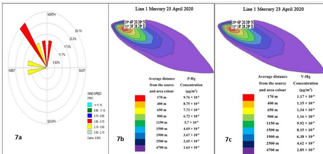
Figure (7): Output of the AERMOD model of line 1 in Helwan area during the day of sampling (April 23rd, 2020) 7a (Wind speed (m/sec) and direction), 7b (Dispersion model of Particulate Mercury emission load in line 1), and 7c (Dispersion model of Vapour Mercury emission load)
