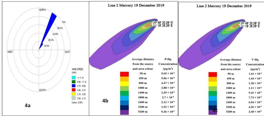
Figure (4): Output of the AERMOD model of line 2 in Helwan area during the day of sampling (December 19th, 2019) 4a (Wind speed (m/sec) and direction), 4b (Dispersion model of Particulate Mercury emission load in line 2), and 4c (Dispersion model of Vapour Mercury emission load)
