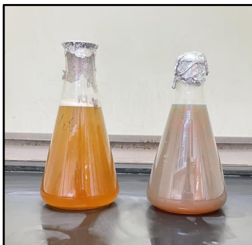
Figure(1): Color change due to the reduction of metal ions and the formation of silver nanoparticles.
