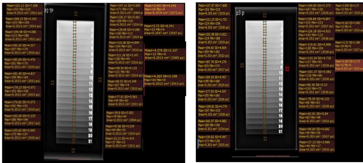
Figure 1. SNR measurement on Stepwedge without and with AHE application
