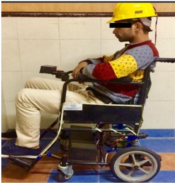
Figure 1. Quadriplegic patient settled on the head movement controlled wheelchair
