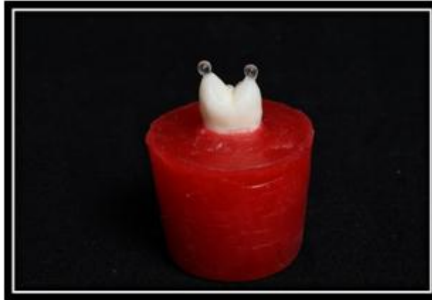
Figure 1: glass beads fixed to cusp tips as reference point
