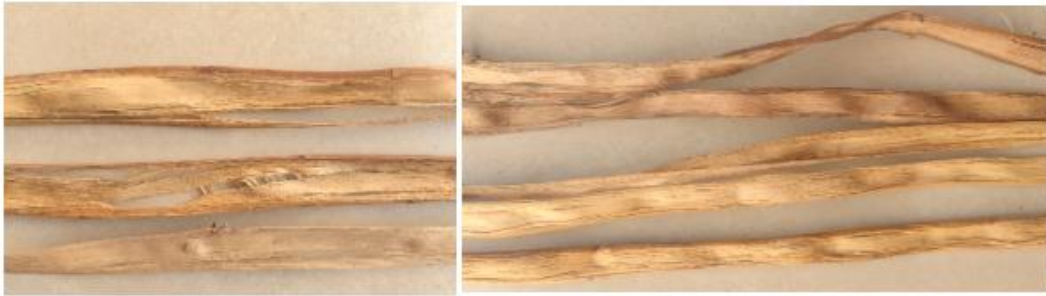
Figure 2: The rattan fiber strips were broken and wavy due to extreme heat during the drying process
