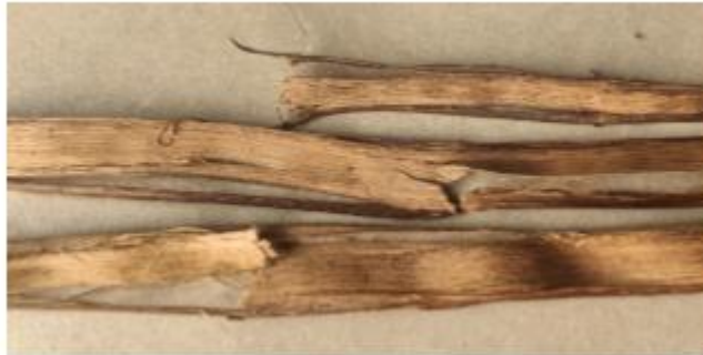
Figure 1: (a) The broken rattan fiber strip while being pressed
