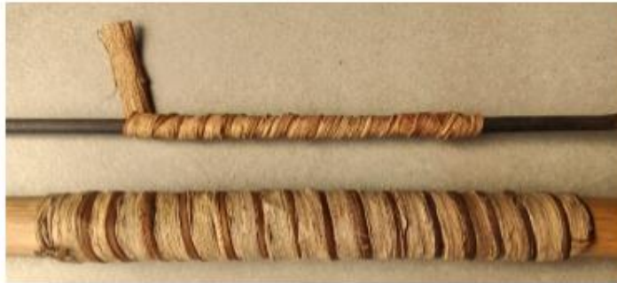
Figure 5: The rattan fiber strips are flexible and applicable to produce products with winding technique
