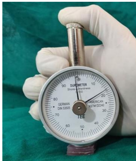
Figure 8: Shore A Hardness Value (Shore A Hardness Number) Being Checked Using Durometer
