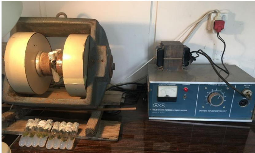
Figure (1): Magnetic field device used for exposure Seed, Explant and Callus cultures
