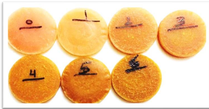
Figure (9) Thermal conductivity test samples before and after the examination
