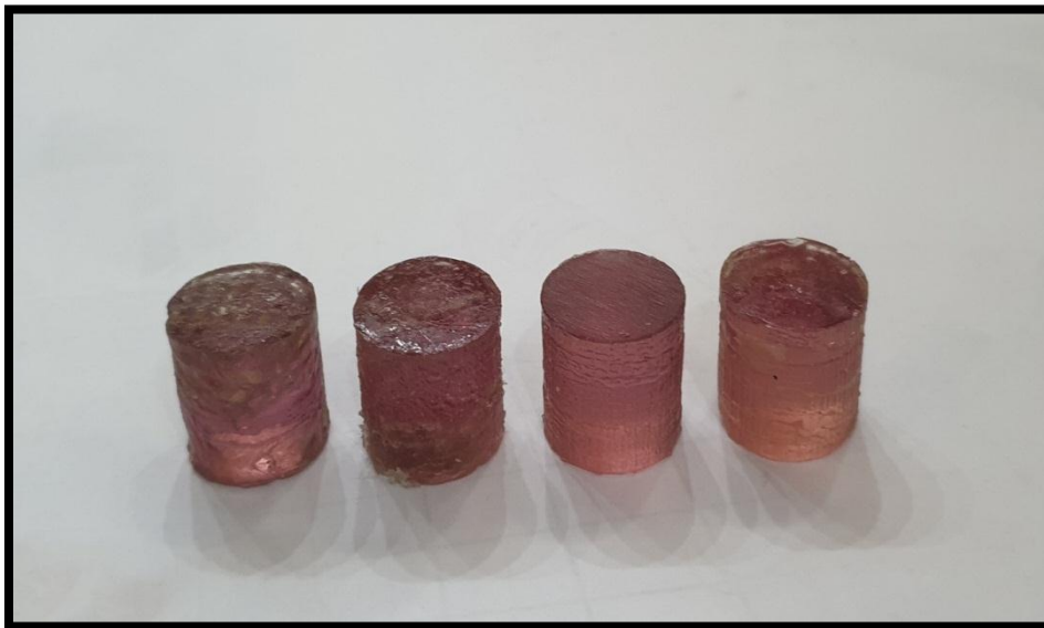
Fig. (2) Shows the shape of the sample prepared for compressive resistance testing
