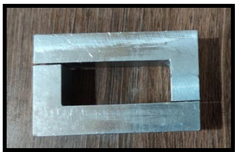
Figure 3a- Custom made rectangular metallic molds
