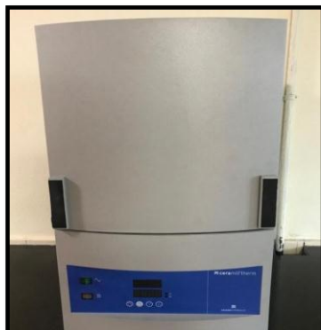
Figure 2a - Sintering furnace (AmannGirbac h Ceramill® therm
