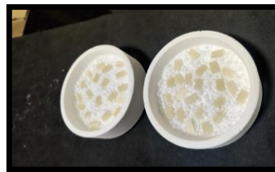
Figure 2b- Zirconia Samples after sintering
