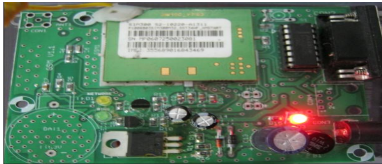
Fig 6: LED glowing indicates the insertion of SIM of card to the GSM modem
