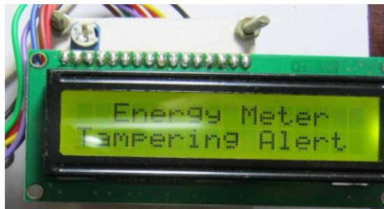
Fig 14: Display showing the tampering of energy meter
