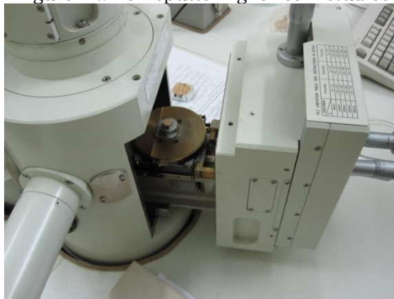
Figure 13. Loading of the sample specimen into the scanning electron microscope
