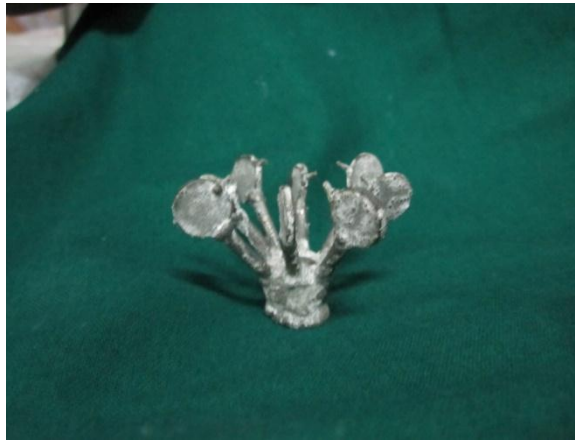
Figure 5. Castings retrieved from the casting ring
