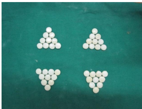
Figure 7. Specimens of metal fuse to ceramic
