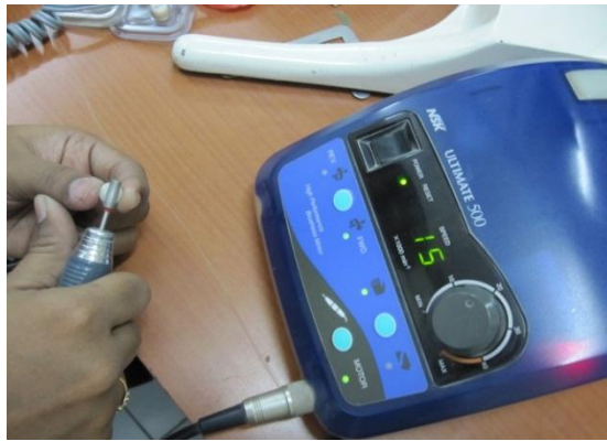
Figure 8. Digital Micro Motor and Hand Piece with sintered diamond bur
