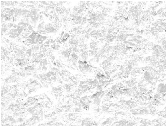
Group II diamond polished sample surface 100 X magnification
