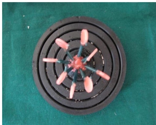
Figure 2. Spruing of specimens
