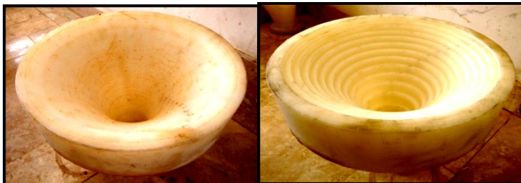
Figure 11. (right to left) simple spillway and 12-step spillway
