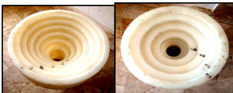
Figure 12. ( right to left) 6-step spillway and 4-step spillway
