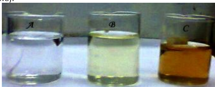
Fig. 2: A. Aqueous solution of 1Mm AgNO 3 ; B. Aqueous solution of 1Mm AgNO 3 with MERN after 0 min; C. Aqueous solution of 1Mm AgNO 3 with MERN after 5 hr.
