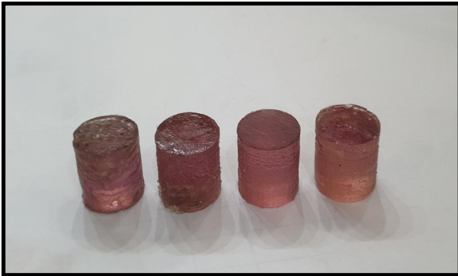
Figure 2: Shows the shape of the sample prepared for compressive resistance testing
