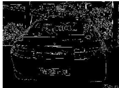
Fig. 2: Applying Filter to find edges and contours
