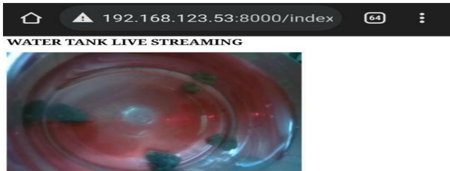
Fig 5. Live streaming of water tank with sediments.
