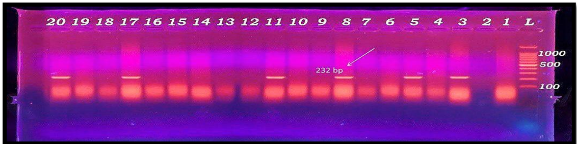
Figure (3-3) Agarose gel with ethidium bromide stained of mono-plex PCR amplified product from extract DNA of P. aeruginosa isolates with bla IMP gene primers , Lane (L) DNA molecular size marker (100-bp ladder) , Lane (3, 5, 8,11,17, 20 ) show positive results
