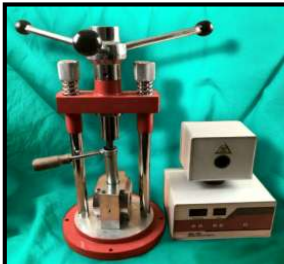
Figure 1. Manual Compression Unit with electric cartridge furnace
