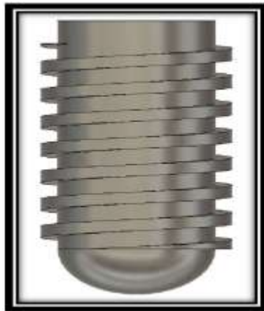
Figure 2: Square shaped Thread of Implant
