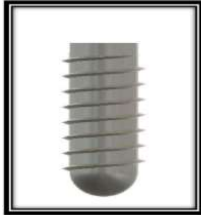
Figure 1: V-Shaped Thread of Implant
