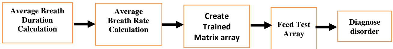
Fig 1. Block diagram of software program development
