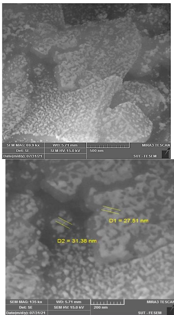
Figure (2): SEM images of Metformin NPs
