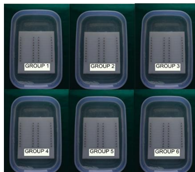
The Jigs with stretched Elastomeric chains dipped in artificial saliva
