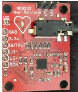
Fig 3. Heartrate monitor sensor
