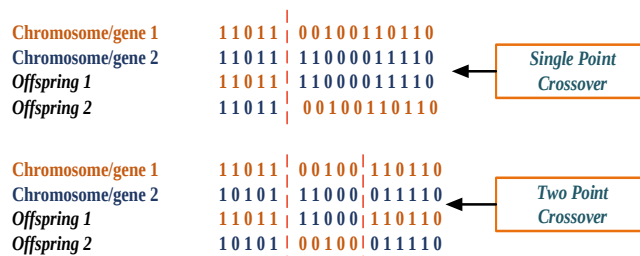
Figure 4. A typical scenario of a single point crossover (top) and two-point crossover (bottom)
