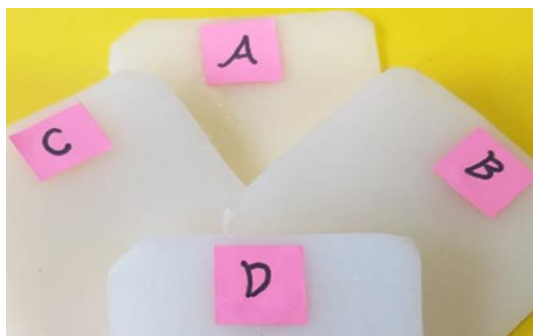
Figure 1. Tissue equivalent specimen produced A, B, C and D paraffin wax-based materials
