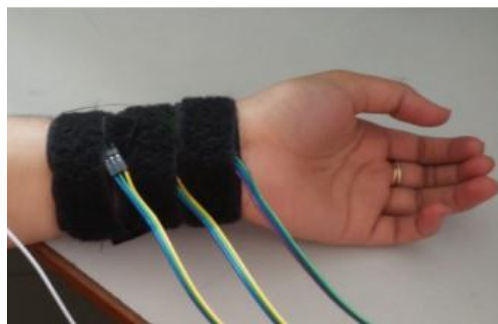
Fig. 2. Placement of PPG sensors on the wrist.
