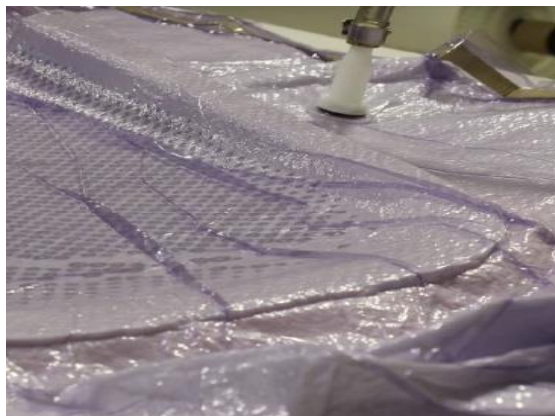
Figure3.2.4 Vacuuming in composite laminates
