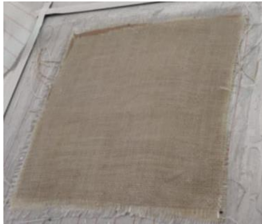
Figure3.2.3 Fabrication of Flax fiber coated composite laminate
