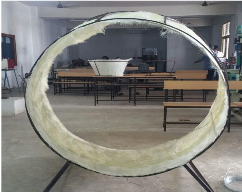
Fig 3.6 Duct Prepared With Composite Material
